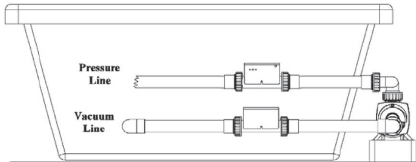
Once the heater is installed, operation is totally automatic. The heater will help maintain the temperature of the water in the bathtub, or increase the temperature of the water in the bathtub at about two to four degrees Fahrenheit per hour. The heater includes the following components.
