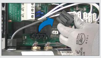
Unplug the heater power connector by depressing the holder clip to release the female connector.
